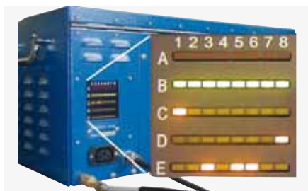
PSS Pro-Service System: Simple functional test with no need to open the unit
