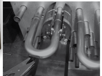
Simple and fast assembly of the weld heads on the tube. Self supporting weld head.
