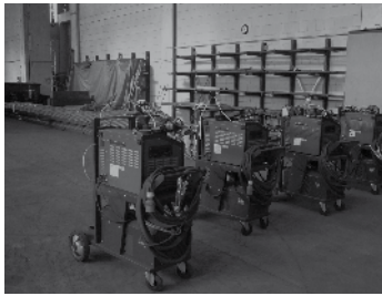
Automatic programming which generates welding parameters by entering the tube diameter, wall thickness, material and welding gas.
