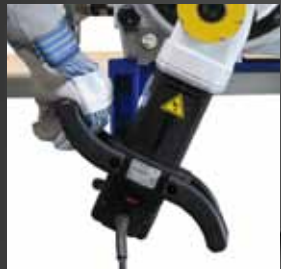
Powerful drive with electronic overload protection and ergonomically designed motor handle
