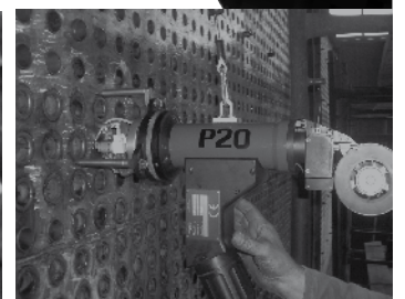
Easy and safe handling with most functionality. Precise centering by means of exchangeable mandrels.
