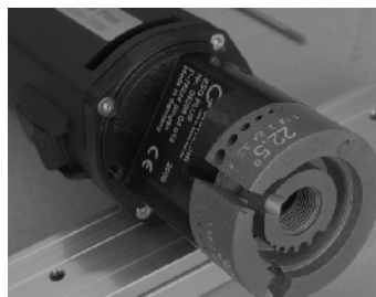
ESG Plus hand-held grinder for cutting, grinding and planing electrodes.
