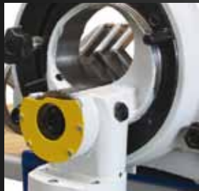
Second saw blade position to cut off elbows
