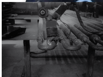
Gas, water and electricity supply through a multiple hose made of viton enables safe and user-friendly working.
