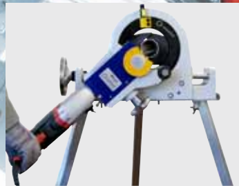
Cutting thin-walled stainless-steel tubes and elbows
