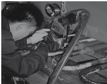
The OP 51 and 102 are also available with electronic arc voltage control (AVC) and oscillation (OSC).
