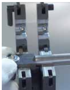
An insertion gage which is permanently attached to the clamping cartridge and thus cannot be lost ensures precise positioning to the tube joint to be welded.
