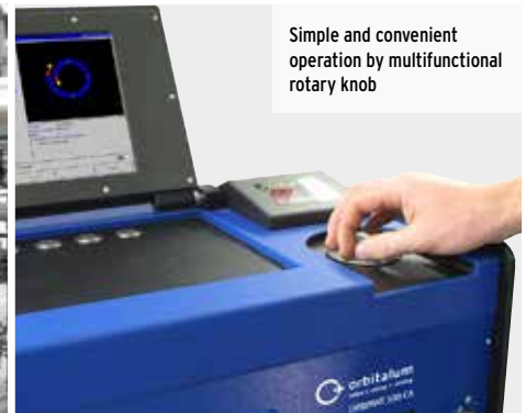
10.5" swivel monitor and system printer integrated
