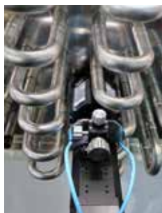
Extremely narrow design - ideal for welding pre-mounted arcs in narrow pipe bundles
